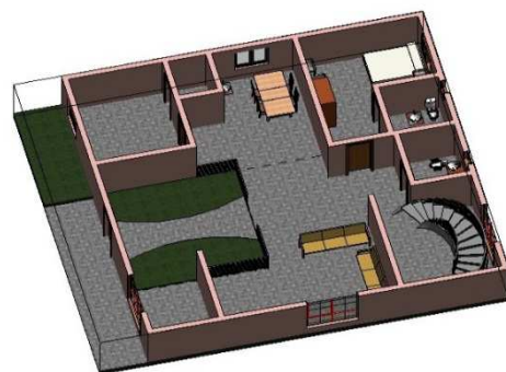
Figure 3: Sectional View of Ground Floor
